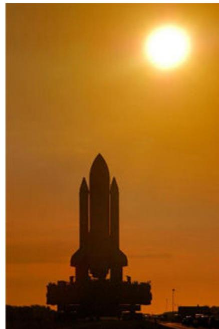
This new design called for a reusable orbiter, reusable rocket boosters, and an expendable external fuel tank. These modifications to the original design cut the cost of the project in half to roughly \$5 billion dollars. What made this new design so extraordinary was that the orbiter would be launched like a rocket, maneuver in orbit like a spacecraft, and be able to land like an airplane.
