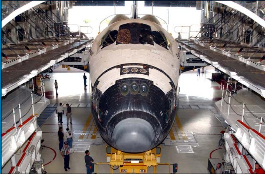
At the OPF, the orbiter is prepared for its next flight. Panels fold down all around the orbiter at the OPF to allow personnel to access the different locations on the orbiter. The Payload may be installed horizontally at the OPF or vertically at the launch pad.
