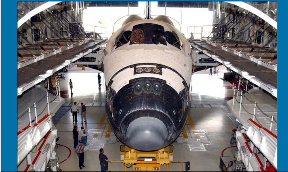
At the OPF, the orbiter is prepared for its next flight. Panels fold down all around the orbiter at the OPF to allow personnel to access the different locations on the orbiter. The Payload may be installed horizontally at the OPF or vertically at the launch pad.
