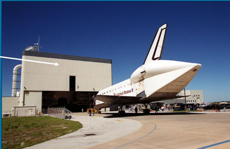
The orbiter is processed at one of three Orbiter Processing Facilities at KSC after landing and before rolling to the VAB for stacking. At the OPF, the orbiter is prepared for its next flight. The Payload may be installed horizontally at the OPF or vertically at the launch pad.
