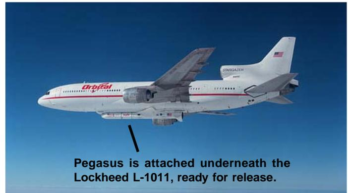
**Pegasus is attached underneath the Lockheed L-1011, ready for release.**
