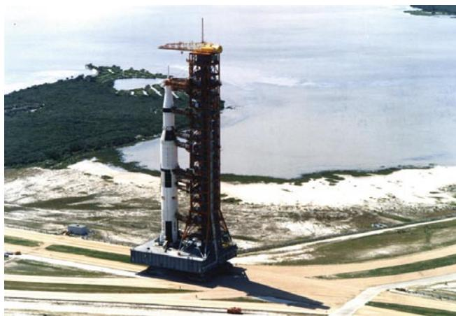
Carrying the Apollo 11 Saturn V space vehicle and mobile launcher, the crawler transporter inches its way to the hardstand on Launch Complex 39A, where it will position the 12.5-million-pound load on support pedestals.
