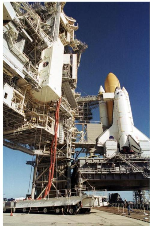
At the launch pad, a payload canister is lifted up the rotating service structure (left) to the payload changeout room. Below, the payload canister transporter maintains the clean environment via the umbilicals (red) still attached.
