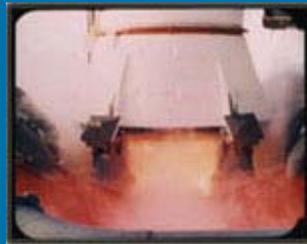
Each SRB has four hold-down posts securing it to the launch platform.
