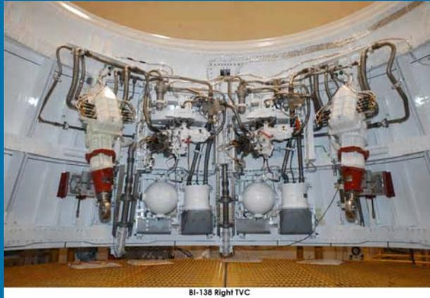
Each SRB has two hydraulic gimbal servoactuators: one for rock and one for tilt. The servoactuators provide the force and control to gimbal the nozzle for thrust vector control.
