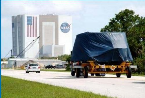
With a Security escort, the first Solid Rocket Booster (SRB) aft skirt for mission STS-114 nears the Vehicle Assembly Building on its transfer to the Rotation Processing and Surge Facility for stacking. At the facility, an aft motor segment and an external tank attach ring will be installed. The stack will then be moved to the Vehicle Assembly Building for further build-up.
