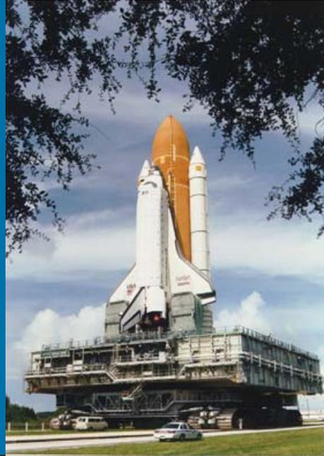
Eight attach posts, four on the aft skirt of each SRB, support and hold the Space Shuttle on the Mobile Launcher Platform. These posts fit on counterpart posts located in the Platform's two solid rocket booster support wells. The space vehicle disconnects from the Platform by explosive nuts that release the giant studs linking the solid rocket attach posts with the Platform support posts.
