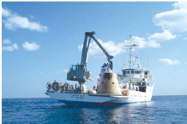
(Left) The frustum is lifted from the water by a power block attached to the ship's deck crane.
