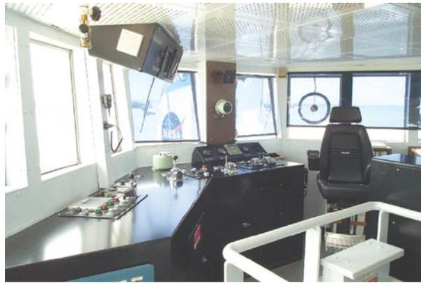
(Left) The forward area of the bridge is for operation of the ship itself. Such state-of-the-art equipment as the Global Positioning System for precise navigation is located here. (Right) Booster retrieval operations are controlled from the aft bridge of the ship. Equipment located here includes hookups for communicating with the divers, forward deck and the other retrieval ship, along with a wind gauge, stern/bow thruster controls and radar.
