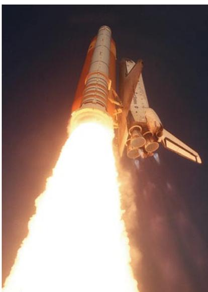
It's a familiar sight during a shuttle launch: When the twin solid rocket boosters (SRBs) have expended all their fuel, they jettison away from the orbiter with help from the booster separation motors, about 26.3 nautical miles above the Earth's surface. They don't fall immediately because their momentum keeps them traveling upward for about 70 seconds, to approximately 38.6 nautical miles. Then they begin their tumble back toward the ocean.
