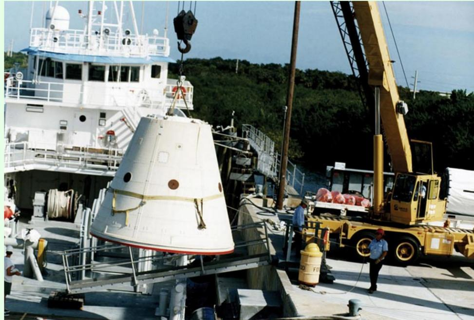
The frustum undergoes extensive inspection, non-destructive evaluation, and repair procedures before the application of protective finishes.
