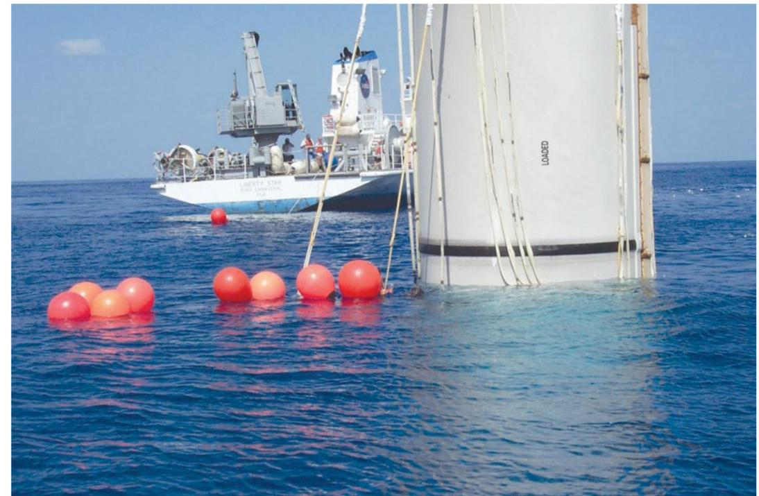
A Solid Rocket Booster Retrieval Ship has arrived on scene after splashdown of an SRB segment following a space shuttle launch. The segment floats vertically until divers can insert an enhanced diver-operated plug (EDOP) into the nozzle of the booster. The EDOP pumps air into the empty casing until all water is expelled and it falls horizontally and can be towed back to port.
