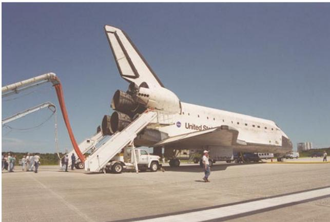
2 Umbilicals are attached to purge the vehicle of any possible residual explosive or toxic fumes.
