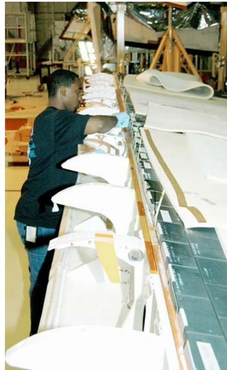
In the Orbiter Processing Facility, a technician prepares the blanket insulation to be installed on the body flap on orbiter Discovery. The blankets are part of the Orbiter Thermal Protection System, thermal shields to protect against temperatures as high as 3,000° Fahrenheit, which are produced during descent for landing.
