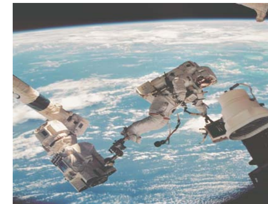
STS-112 Mission Specialist David A. Wolf is anchored to a foot restraint on the Canadarm2 as he carries the Starboard One (S1) outboard nadir external camera to the S1 Truss on the International Space Station.
