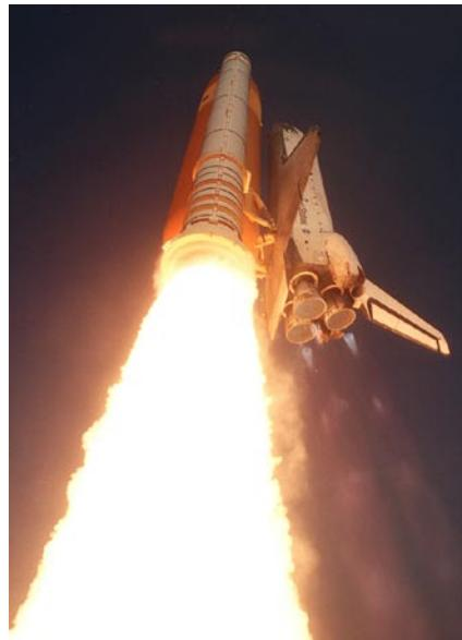
ers. As in the case of hydrogen, shuttle servicing requires more oxygen than the actual capacity of the oxygen compartment. About 250,000 gallons (2,580,000 pounds) are used in all.
