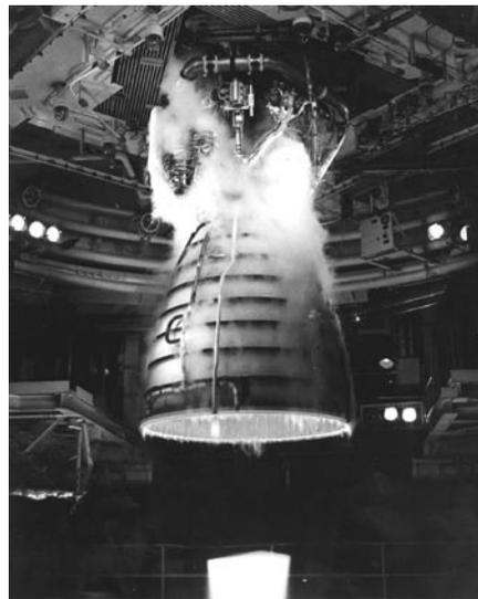
Shuttle main engine test firing at Stennis Space Center in Mississippi
