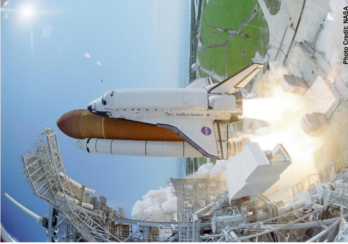
At about T minus 4 minutes, 55 seconds, the liquid oxygen vent on the external tank is closed. It had been open to allow the super-cold liquid oxygen to boil off, thus preventing over pressurization while the tank remained near its full level. Now, with the vent closed, preparations are made to bring the tank to its flight pressure. This occurs at T minus 2 minutes, 55 seconds.
