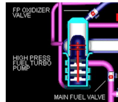
SSME console next to the HPFTP or HPOTP. You can calculate the amount of mass coming out of the HPFTP or HPOTP by multiplying the maximum flow rate by the percentage the valve is opened.
