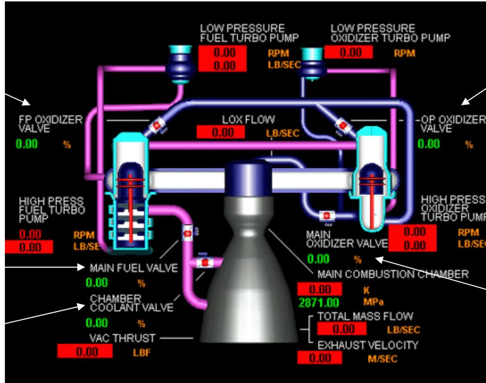
OP Oxidizer Valve controls Oxidizer (LOX) to the HPOTP
