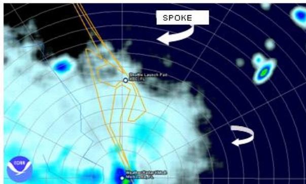
1. The range rings start 10 miles from Melbourne moving out toward the KSC Launch Pad.
