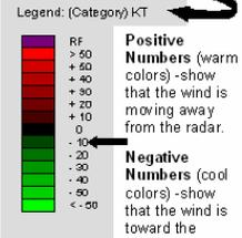
Velocity - This product is used to estimate wind speed and direction.
