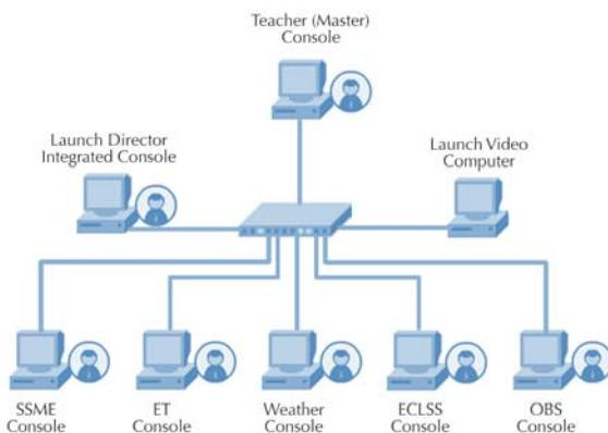
There are quite a few possibilities for setting up the simulation lab. There are 5 different KCLASS student consoles. The SSME console is designed for 3 SSME engineers. In addition, the weather console has a primary view and 4 different views. There is also an integrated view that shows a summary of all systems. Ideally, an integrated simulation set-up could include these items:
